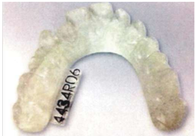
Figure 12. Stereo lithography model
